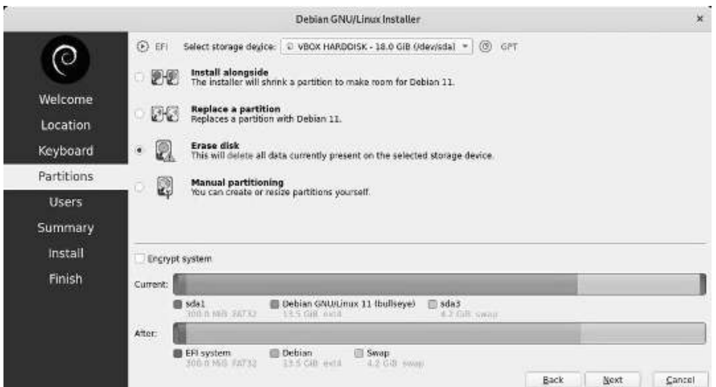
Calamares installer : partition scheme
