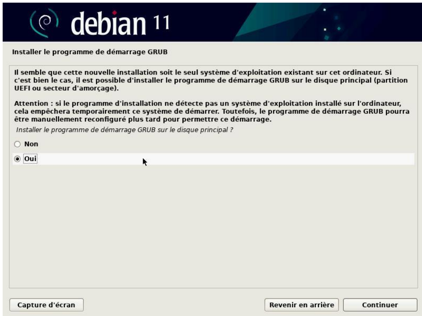
Installation : installation de GRUB
